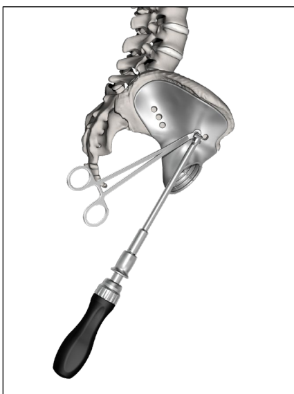
Figure 25: Use of Screw Forceps to hold screw head while inserting with In-line Ratcheting Modular Handle and Flexible Bayonet Driver (Left). Use of Screw Forceps to hold screw head while inserting with In-line Ratcheting Modular Handle and Universal Joint 3.5mm Hex Driver (Right).
