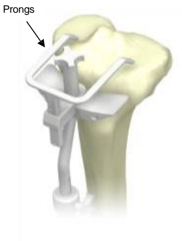
Adjust prongs of tibial cutting guide to sit on the plateau of the tibia
