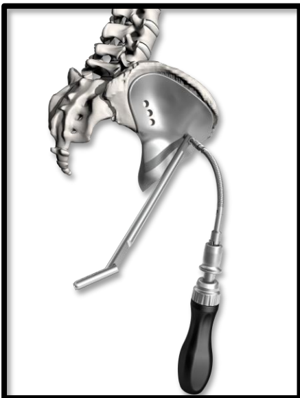
Figure 19: 25mm bayonet drill with flexible driver and drill guide can be used to predrill holes in ischium, pubis, or any other area where a straight drill cannot easily access.
